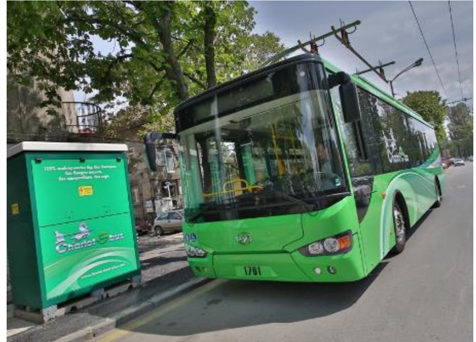
*Why not to use supercaps to power the buses between stations and recharge the caps during the time passengers are getting on and off the bus?*
